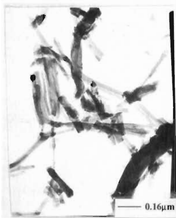
Figure 1. Transmission electron micrograph of the solid product formed upon reacting [EtZn(SBu^1)]_2 with H_2S at a flow rate of 5 cm 3 /min in CH_2Cl_2 solution at 22 °C.
